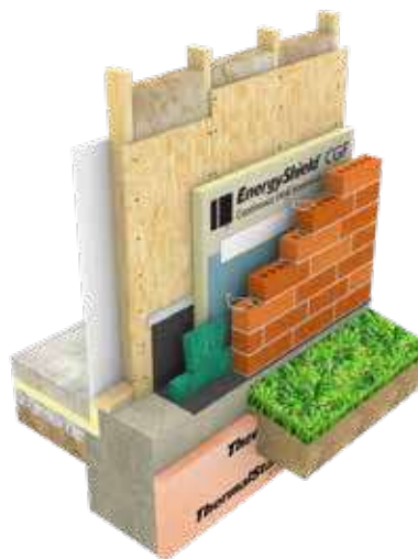
Wood studs, batt cavity insulation, wood sheathing, EnergyShield CGF, liquid applied air and moisture barrier, mortar net, brick.
